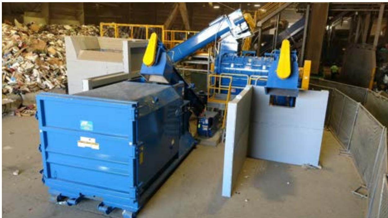
Figure 16. Organic Pre-processing Facility. The Mega THOR Turbo Separator effectively separates contamination from the food waste stream
